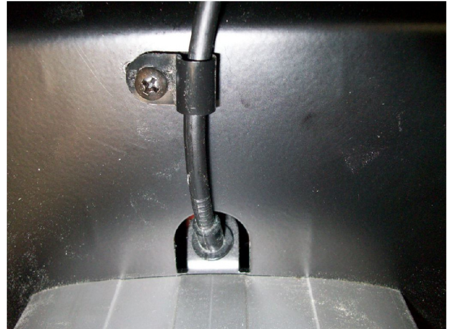
RELEASE CABLE SHOWN EXITING THE WORKSURFACE SUPPORT STRAIGHT
