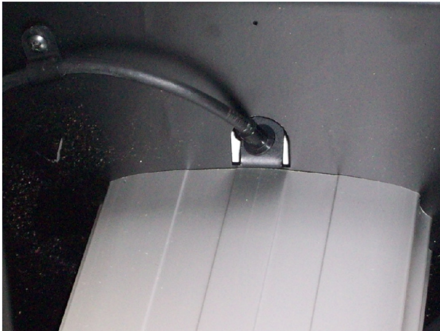
RELEASE CABLE SHOWN EXITING THE WORKSURFACE SUPPORT AT AN ANGLE
