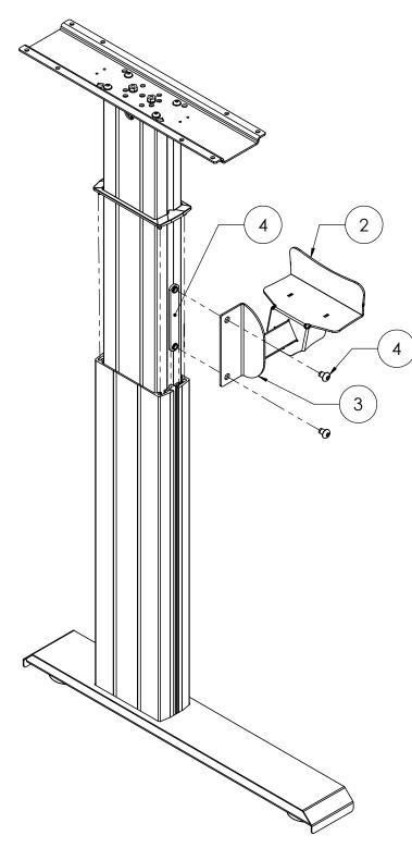
**Step 5:** Place your CPU onto CPU holder Assembly B <u>1</u> and slide the support bracket <u>2</u> tightly against the side of your CPU.
